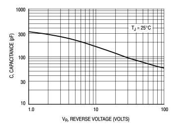
Figure 10. Typical Capacitance
