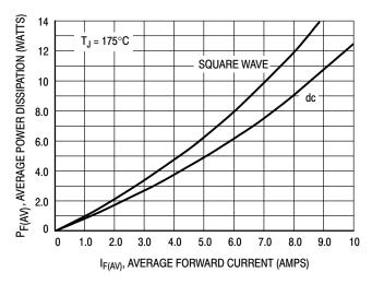
Figure 5. Power Dissipation
